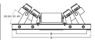
It is important to ensure that adequate power is available in the conveyor drive to compensate for additional frictional drag when installing one or more Warrior Slider Beds.
